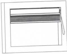
The middle rail and bottom rail will go down together when you operate following the direction of the red arrow
