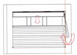
5) When you continue to operate the cord following the direction of the red arrow, the bottom rail and middle rail will go up together once the middle rail gets to the bottom
